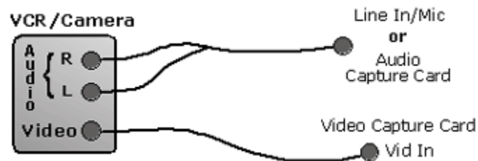
Figure 6: Connecting a VCR to a video capture card.
